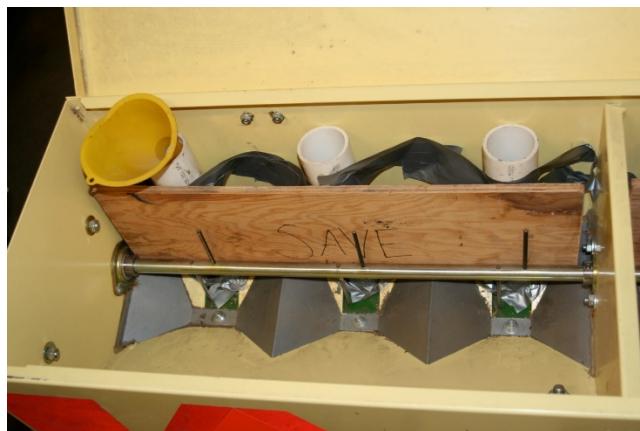
Figure 3. Seed drill modification for planting small areas
