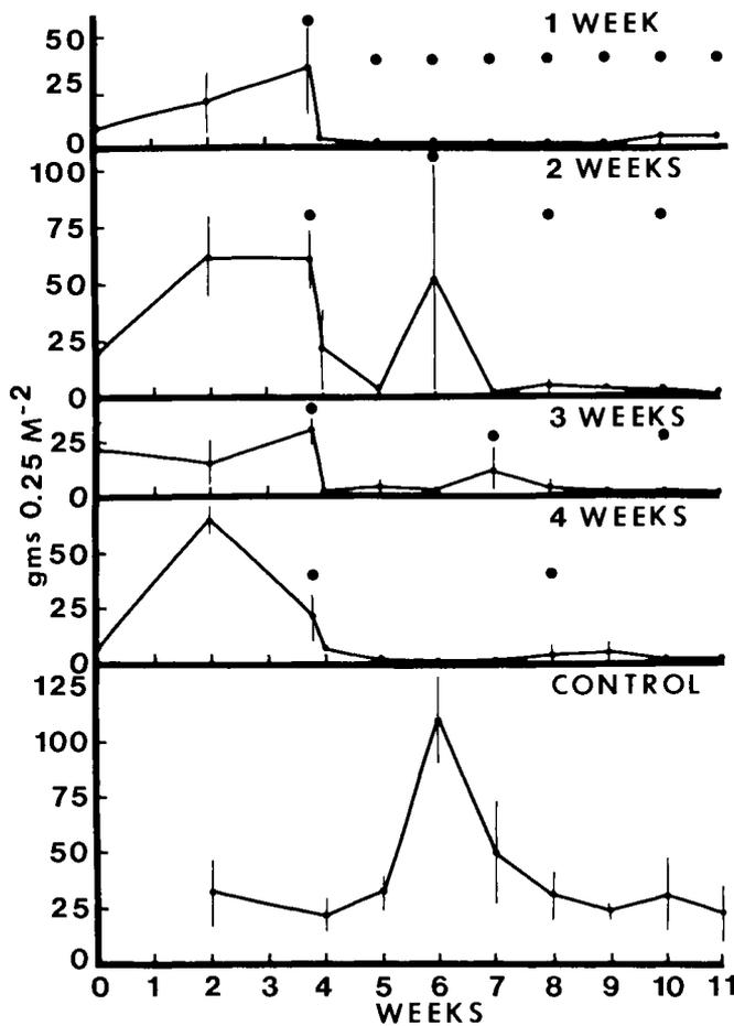
Fig. 4. The effect of harvest frequency on regrowth of aquatic macrophytes in LaDue Reservoir. Dots indicate times of harvest. Data are gms. dry wt. 0.25 m<sup>-2</sup>. Bars are +/- one standard error (redrawn from Cooke and Carlson, 1986).
