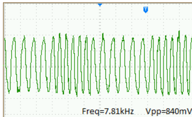
Figure 25. FSK Signal Obtained between the Left Earphone Channel and the Ground
