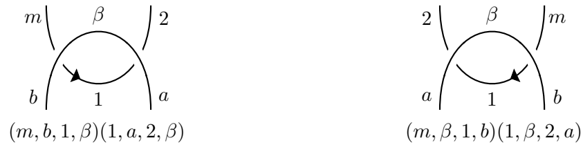
Figure 2.13: Knot segment diagrams with consecutive PD code tuples of the form (m, b, 1, \beta)(1, a, 2, \beta) and (m, \beta, 1, b)(1, \beta, 2, a)
