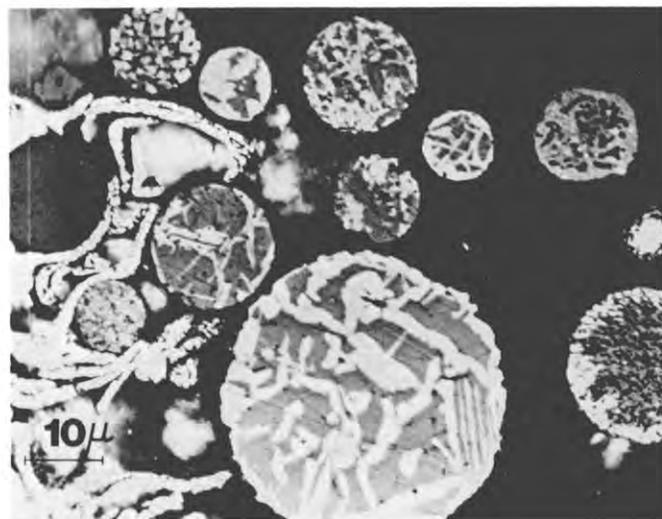
Figure 6. Photomicrographs of the cross-sections of particles from the magnetic fraction of fly ash.
