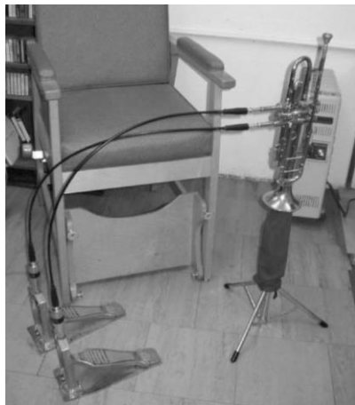
Figure 16: Foot adaptive trumpet
