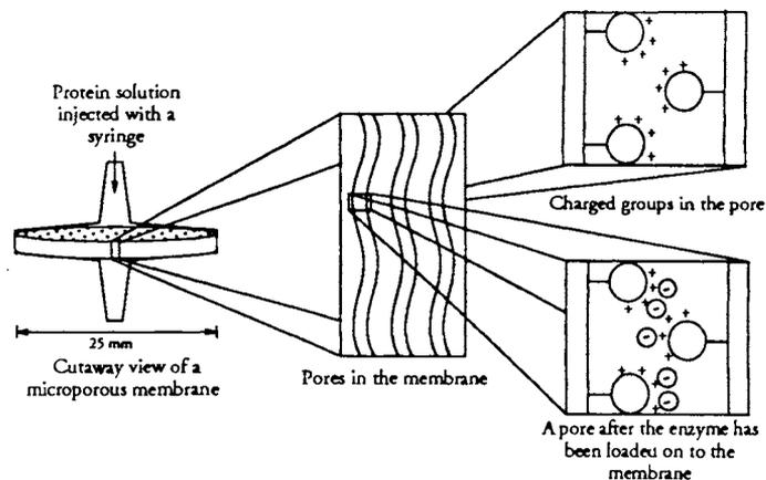
Fig. 1. Schematic diagram of a microporous ion-exchange membrane.
