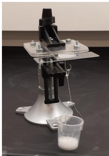
Figure 2: Apparatus used to measure adhesive strength.
