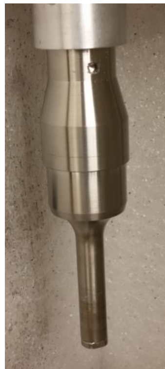
Figure 1: Probe used during the ultrasonication process to create the suspensions.
