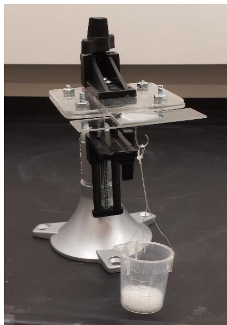
Figure 2: Apparatus used to measure adhesive strength.
