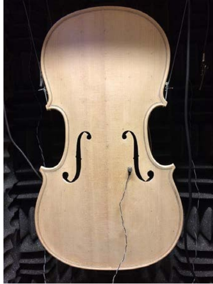
Figure 2. Spruce wood unattached violin front plate hung in the soundproof chamber with the micro-accelerometer attached for vibrational analysis.
