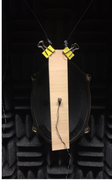
Figure 3. Spruce tone wood strip hung in the soundproof chamber with the micro-accelerometer attached for vibrational analysis.
