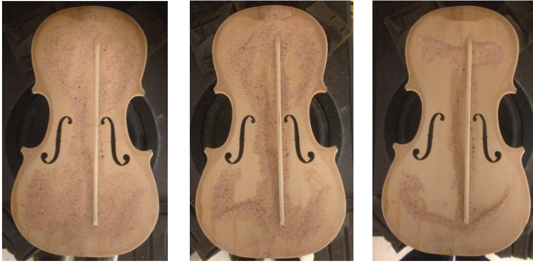
Figure 9. Images of the normally-carved unattached violin front plate with Chladni lines. From left to right, the initial sand scattering, 230 Hz Chladni line, and 340 Hz Chladni line.
