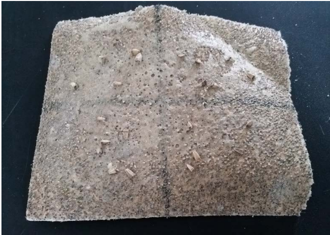
Figure 10: Seed card design showing sandpaper, divided into four quadrants, and seeds between layers of aerosol adhesive.
