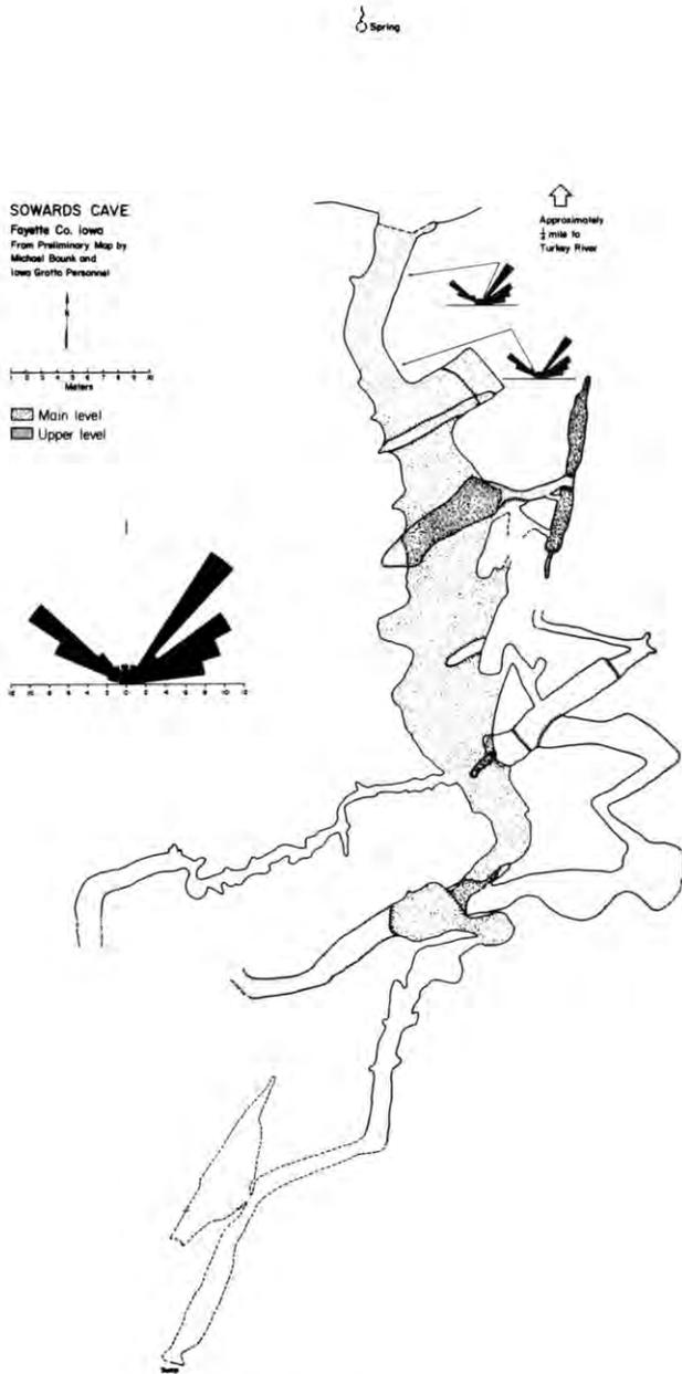
Figure 9. Map of Sowards Cave, showing the relationship between a rose diagram based on surface rock joints, ground-water gradient (downhead to the north) and cave morphology.
