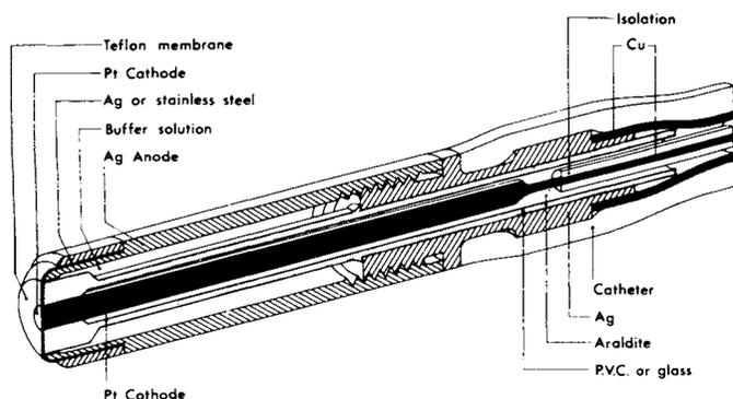
Fig. 1 The Kimmich-Kreuzer catheter oxygen-electrode. It has a single wire cathode ( $400\mu$  in diameter) for use in the gas phase (Kimmich, H.P., 1969).
