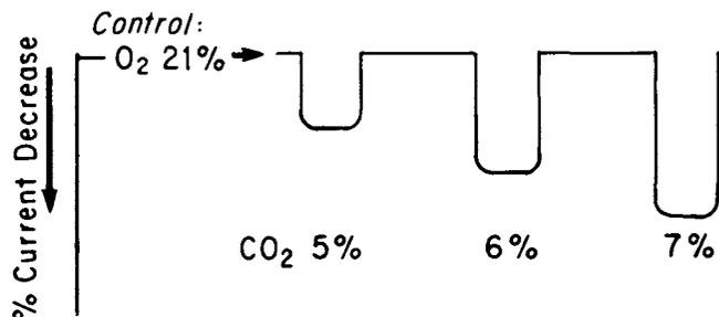
Fig. 2 Conceptual chart recording of the error in the catheter  $pO_2$  electrode in the presence of  $CO_2$  mixtures.
