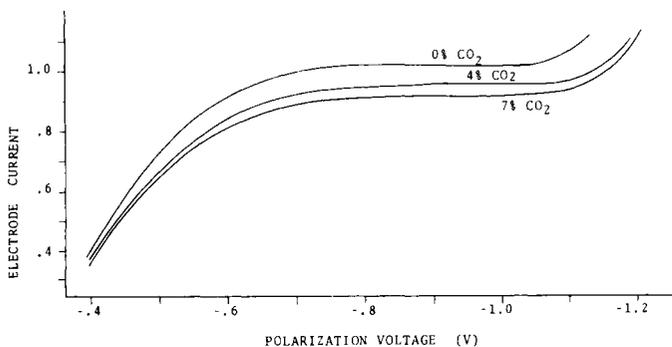
Fig. 3 The effect of CO<sub>2</sub> on the 21% O<sub>2</sub> polarogram. An X-Y recorder was used.
