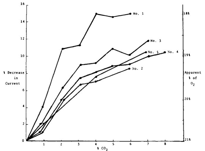
Fig. 4 Five replicates on successive days with different membranes from catheter pO<sub>2</sub> electrode using a chart recorder with 21% O<sub>2</sub> and variable CO<sub>2</sub> mixtures. These results fall within calculated lines for 95% confidence limits for the linear and the quadratic regression models.
