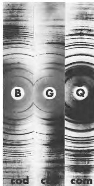
Fig. 2. X-ray diffraction patterns for two hydration forms of Ca oxalate; cod = dihydrate (weddellite); com = monohydrate (whewellite). Three patterns are from crystals of Begonia sanguinea = B; Geastrum minus = G (Collection B); Quillaja sp. = Q.
