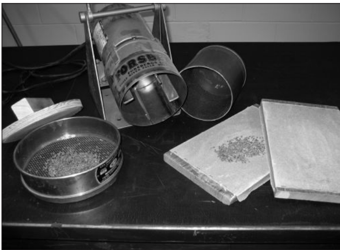
Various equipment for scarifying small quantities of seed. From left to right: Brass soil sieve with sandpaper covered wood paddle, Forsberg scarifier, sandpaper covered wood boards.
