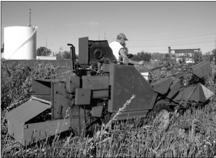
1977 Hege 125B plot combine modified for harvesting native species. Harvesting Rigid goldenrod in this photo.
