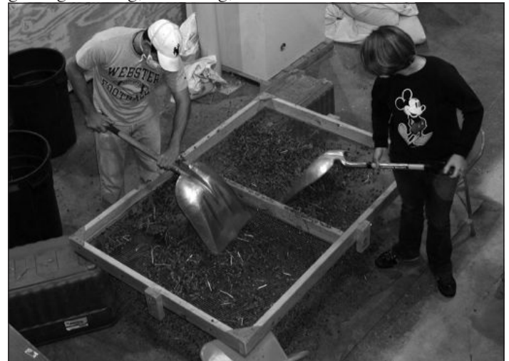
Rough screening combined material through 1/2” hardware cloth to remove large stems and leaves.
