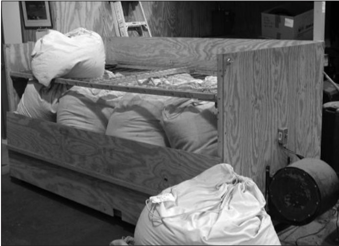
Wooden drying bin with racks for drying bulk bags. Squirrel-cage blower provides ambient air flow.
