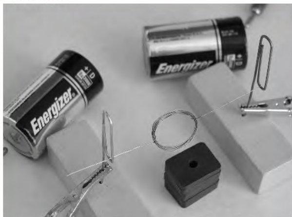
A single coil motor is used to demonstrate the direction of a force.
