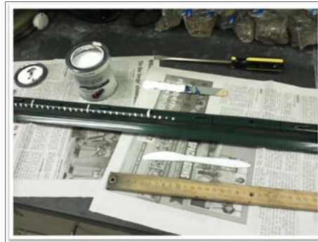
Figure 17. Photo of painted fence post gauge mid-construction.
