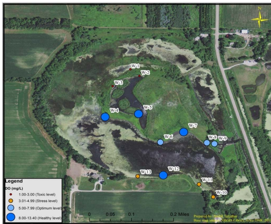
Figure 33: Spatial distribution of average DO at each site during the study period
