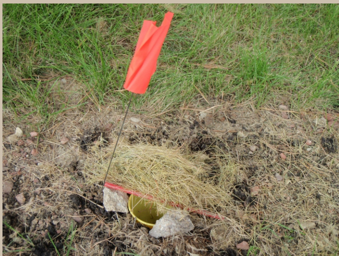
Pitfall trap for crawling insects, complete with marker flag and a cover that's inviting to insects.
