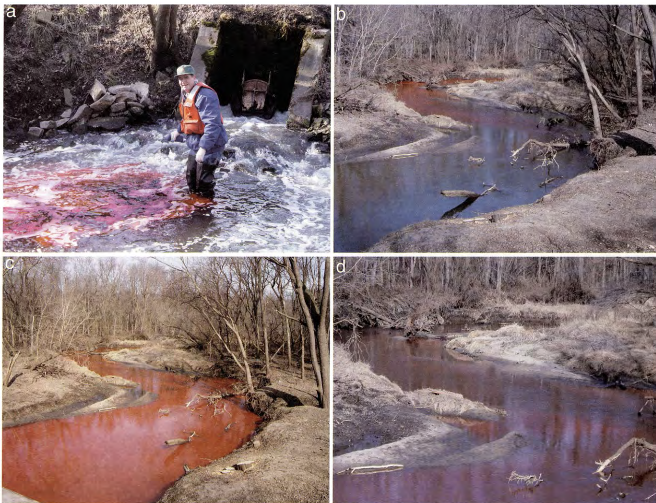
Fig. 3a. Injection of dye at Fourmile Creek near Ankeny, Iowa at the wastewater treatment plant outfall, March, 2005. Fig. 3b. Leading edge of the dye concentration at Fourmile Creek near Ankeny, Iowa, site 3, March 2005. Fig. 3c. Peak dye concentration at Fourmile Creek near Ankeny, Iowa, site 3, March 2005. Fig. 3d. Trailing edge of the dye concentration at Fourmile Creek near Ankeny, Iowa, site 3, March 2005.
