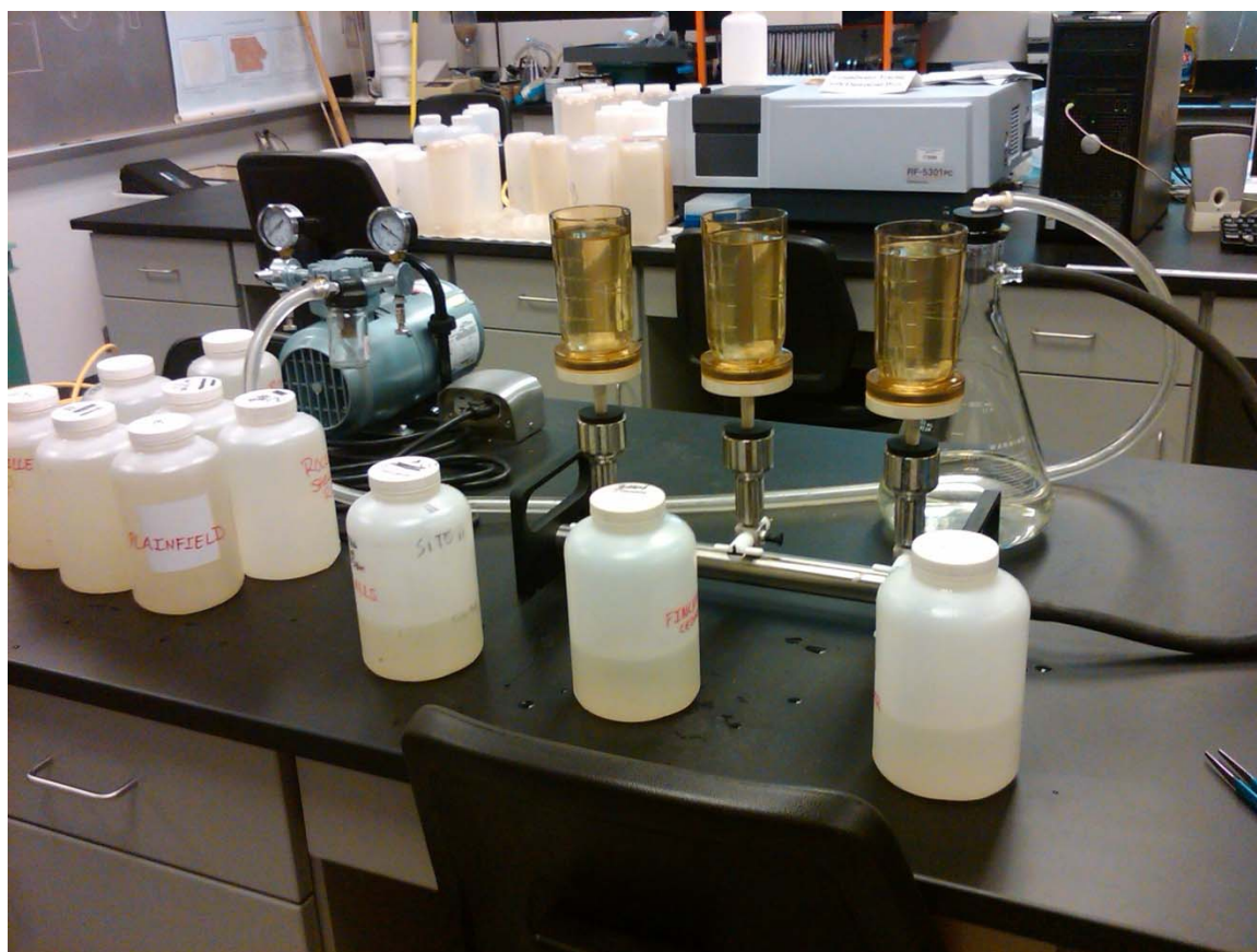
Figure 16. Vacuum pump apparatus used to filter the sample water to calculate suspended sediment.
