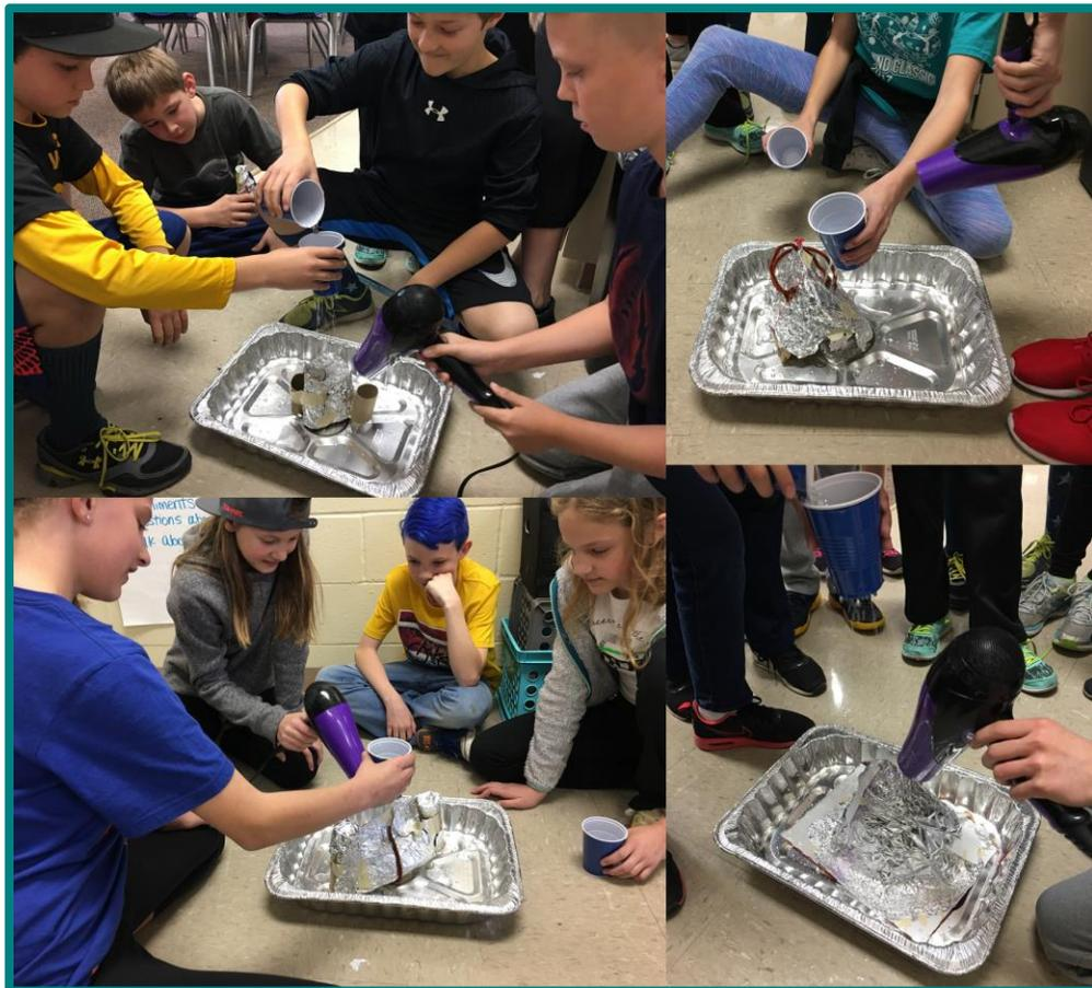
Figure 3. Fifth graders testing their hurricane shelter structures with pouring rain (water from cup) and blowing wind (hairdryer air). In the top left photograph, cardboard tubes were used to balance the shelter during the extreme wind. In the top right photograph, students used pipe cleaners to collect and guide the downpour or rain.
