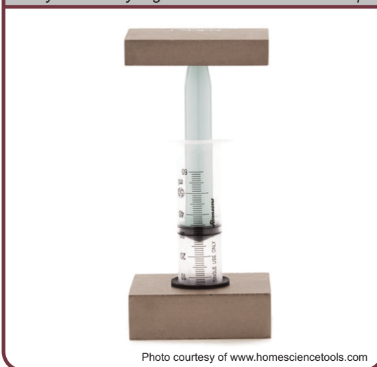
FIGURE 1 Boyle's Law syringe with wooden base and top.
