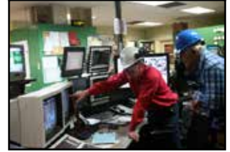
Cedar Falls Utility employees monitor a test burn of pelletized prairie biomass from the Prairie Power Project site.
