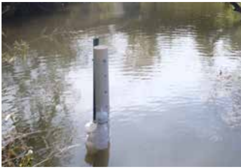
A "stilling well" holds a pressure transducer. This device measures stream stage in 15-minute increments.
