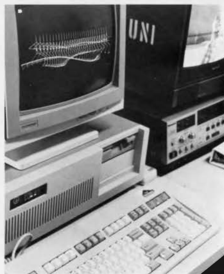
On display, the 2D Video/Computer Motion Analysis System breaks down the movement of a runner. Photo by Veronica Koh.
