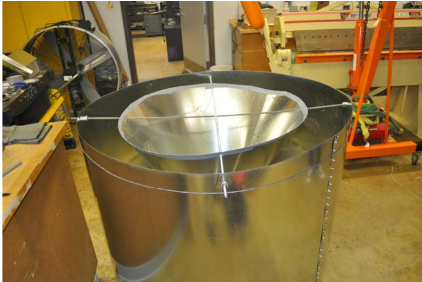
Figure 10. Stabilization of Wind Guide Attachment
