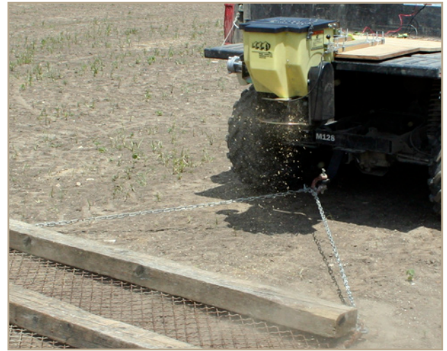
Broadcast sow and rake rig demonstrated on an ATV.
