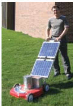
EIET students led by Recayi Pecan (above) designed and built this solar-powered lawn mower.
