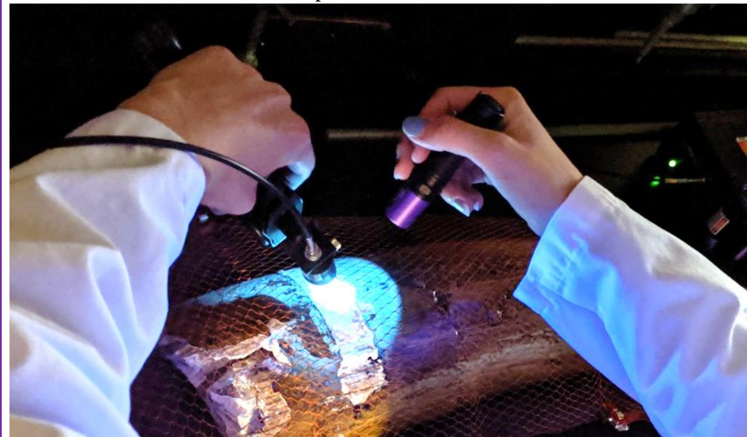
Figure 2 - Fiber Optic Set-Up Used to Gather Fluorescence Spectra
