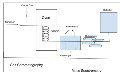
Diagram of GC/MS Instrument
