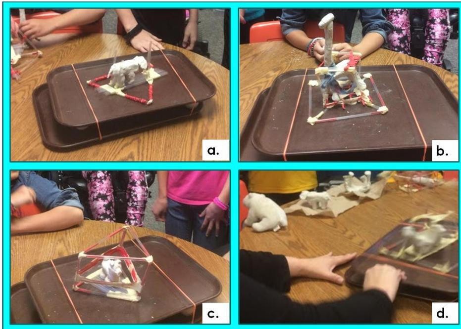
Figure 3. Student work being tested in support structures on the shake table. Figure 3a shows a puppy sculpture being tested; 3b shows the giraffe sculpture that broke apart during testing; 3c shows a pig sculpture that survived the simulation; 3d shows the table in motion.
