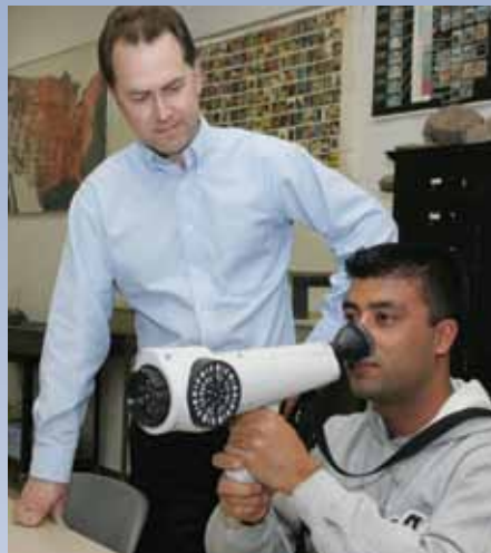
Graduate student Keshab Simkhada demonstrates how to use a field olfactometer in an exercise on odor measurement, as Alan Czarnetzki looks on.
