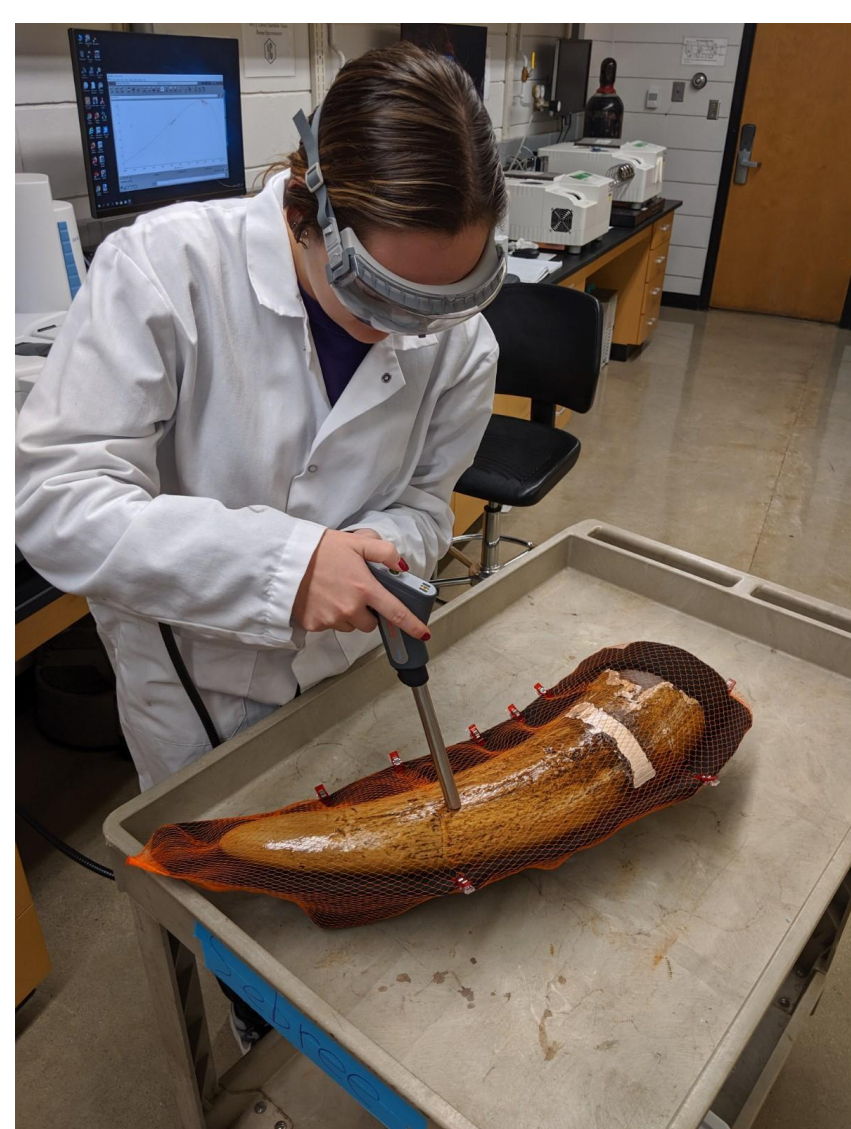
Image 2 Using the SabIR probe on the tusk
