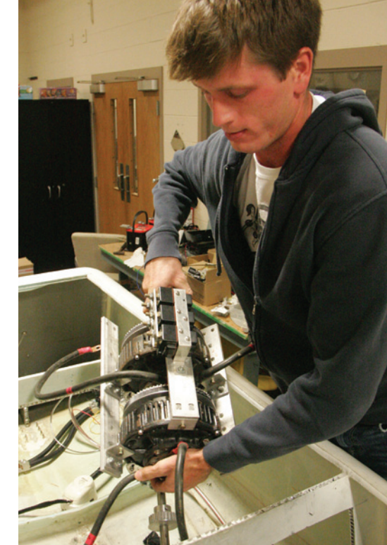
Senior David Buseman installing the UNI solar boat's high-current motor pack.
