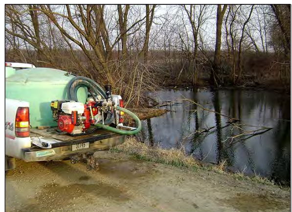
Top: A 400-gallon spray rig equipped with a centrifugal pump and a 300-foot hose. Bottom: Back-up water can be drawn from nearby water sources with a trash pump.
