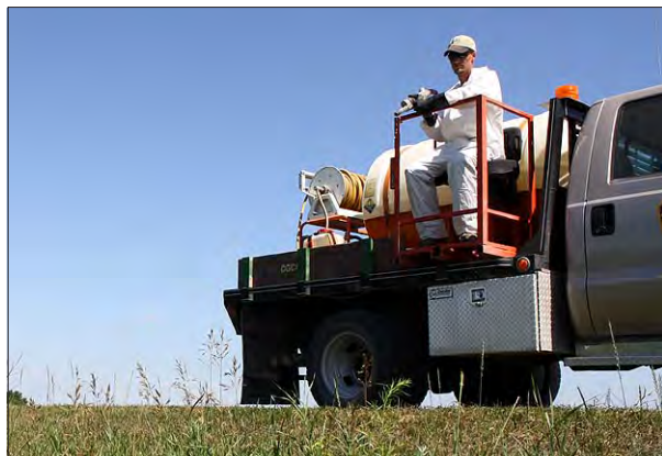
This truck is equipped with an exterior seat for more accurate spraying.
