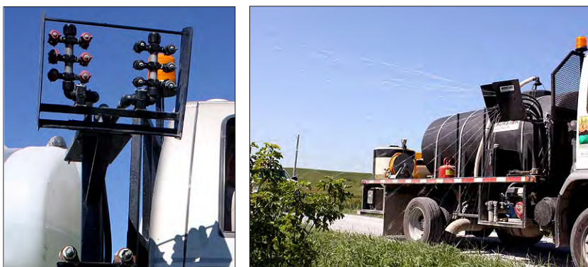
Nutating spray head (left) and spray pattern with all nozzles on (right). Nutating spray heads use banks of solid-stream nozzles that move rapidly in a vertical plane and produce larger droplets, potentially reducing off-target drift.
