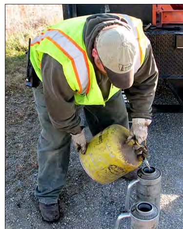
Drip torches are filled with pre-mixed fuel a safe distance from the fire line.
