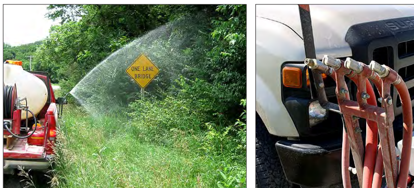
Traditional bumper-mounted nozzles (right) and spray pattern (left). Bumper-mounted nozzles produce smaller droplets and a wider spray pattern.
