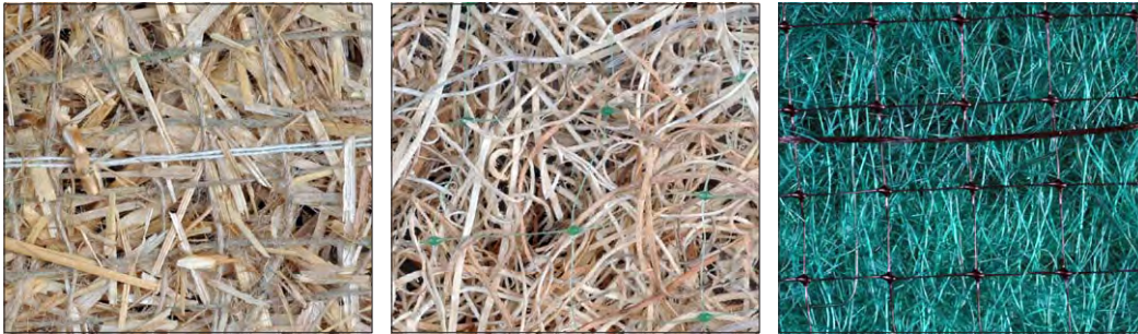
Straw ECB with biodegradable jute netting (left) and excelsior ECB with photodegradable synthetic netting (center). Netting and fiber components, along with site conditions, determine ECB longevity. TRMs (right) provide permanent reinforcement with a matrix of UV-stabilized, synthetic fibers and netting. Level of reinforcement is determined by material and product weight. (Photos courtesy Western Excelsior)
