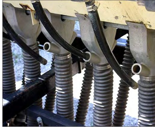
Disconnecting every other tube from the small seed box allows seed to be scattered more naturally and prevents the smaller seed from being buried too deep.
