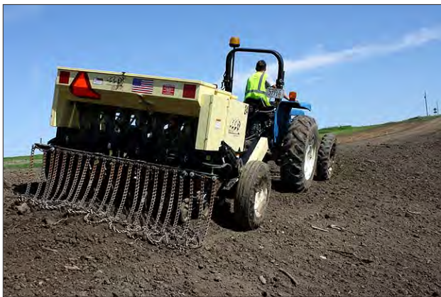
A native seed drill is still the seeder-of-choice for many roadside managers. This one has been modified by the county; drag chain has been added to smooth over seeded area.
